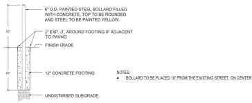
5 STEEL BOLLARD (DETROIT GSD STANDARD) SECTION
