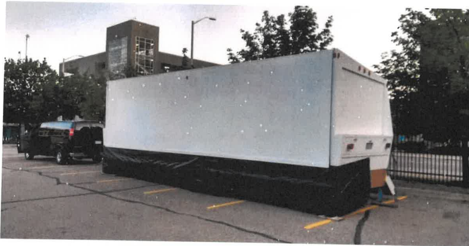
32' Showmobile Portable Stage Has stage lighting,,electrical outlets and 40 amp panel.
