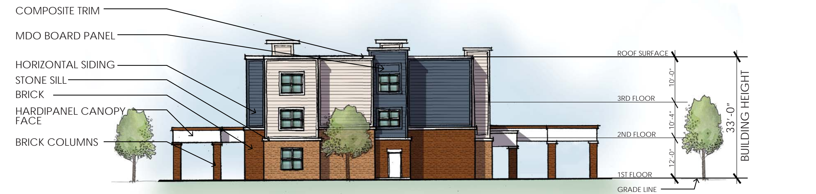
TYPICAL RIGHT SIDE ELEVATION APARTMENT BUILDING
