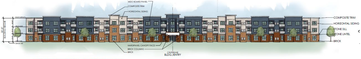
FRONT (STREET) ELEVATION APARTMENT BUILDING 1/16" = 1'-0"
